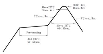
1. Avoid any external stress applied to the resin while the LEDs are at high temperature, especially during soldering.
